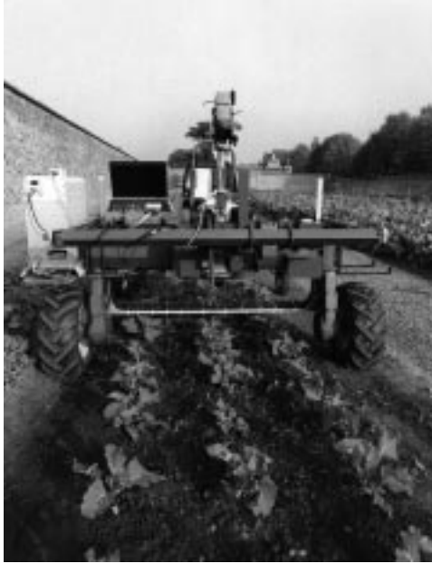
Figure 4. (a) Autonomous vehicle guided by a video camera. (b) Image of cabbages in infrared with the line of rows fitted by analysis.
